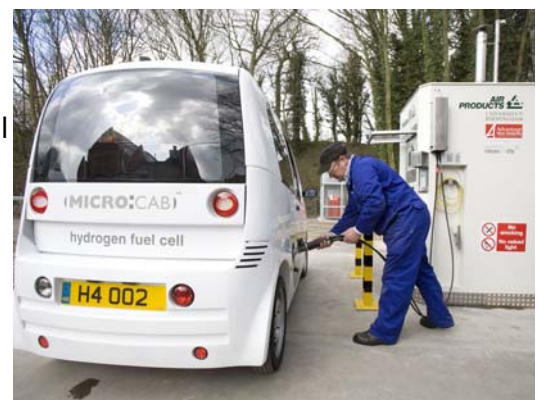
Hydrogen Fuel Cell Hybrid Vehicle being refueled at The University of Birmingham campus
